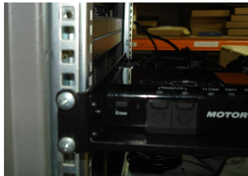
Figure 16: Tray Attached (Left End Shown)
