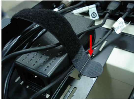
Figure 12: Power Supply Secured
