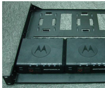
Figure 8: KMF CryptR Units Mounted on Tray
