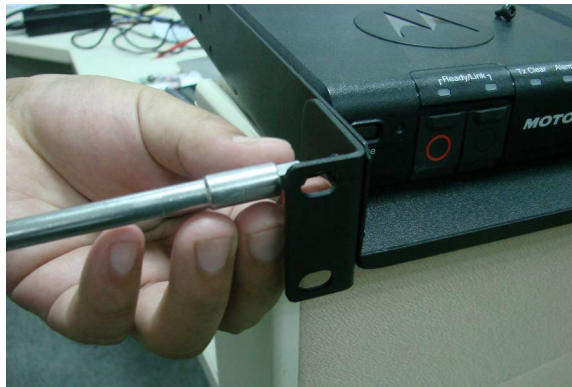
Figure 7: Attaching Supporting Brackets
