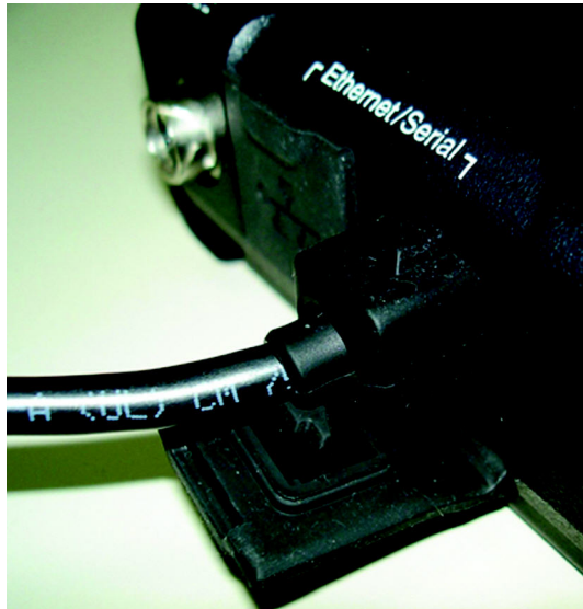
Figure 11: Attaching Ethernet Cable to KMF CryptR
