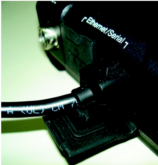
Figure 11: Attaching Ethernet Cable to KMF CryptR
