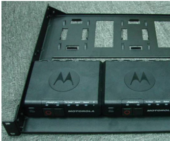
Figure 8: KMF CryptR Units Mounted on Tray
