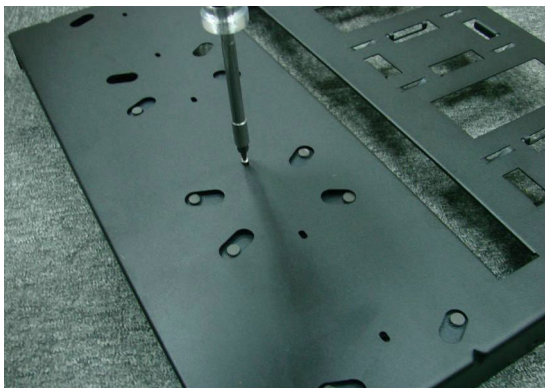
Figure 6: Inserting Mounting Screws Into Tray
