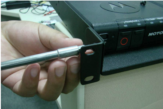
Figure 7: Attaching Supporting Brackets
